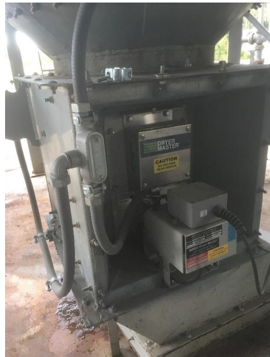
Figure 18 - In-Line chute in a Zimmerman chute
