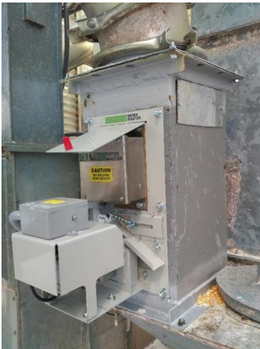
Figure 19 – In-line Chute installation example
