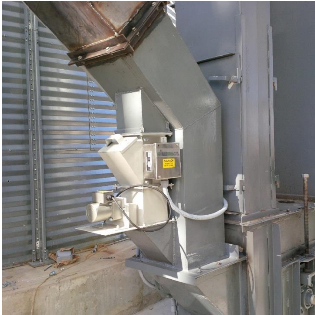
Figure 12 - Example installations of bypass chute with rotary metering
